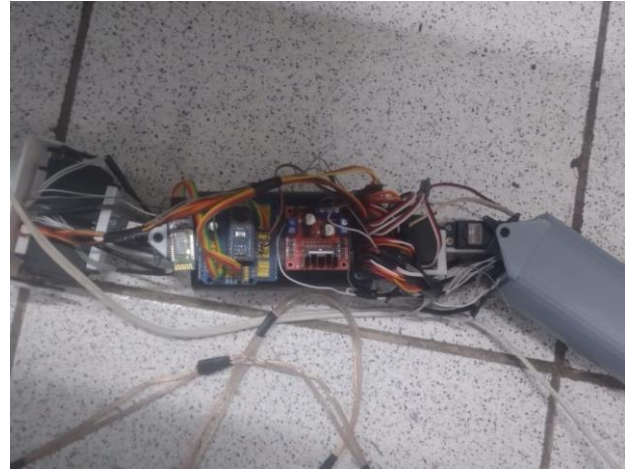
Figure 11. Control unit (Arduino, controller and modules.)
