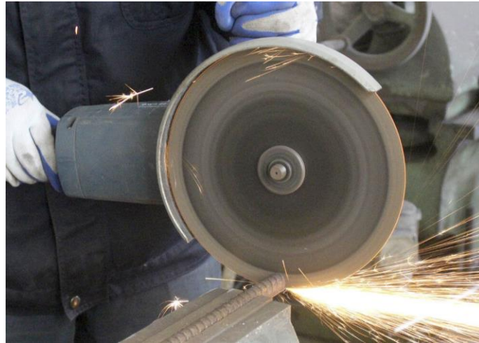
Figure 3: Placing the tube on the base and cutting
