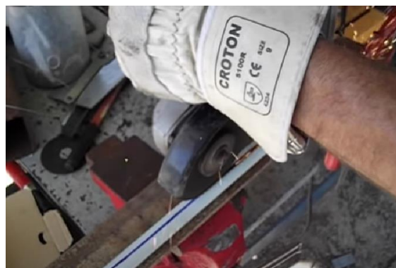
Figure 4: Cut of the tube trace
