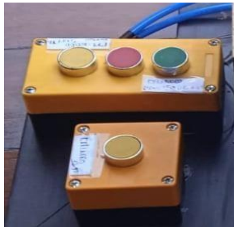
Figure N° 20. Three-button pushbutton Source: Own elaboration
