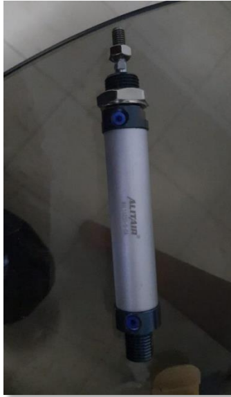
Figure N° 15. 16*50mm double-acting cylinder
