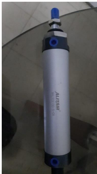
Figure N° 16. 32*100mm double-acting cylinder
